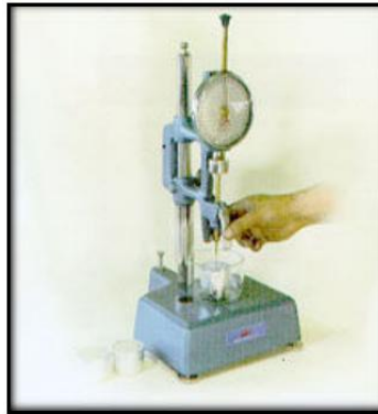
Figure 1. Equipment for determining the penetration.
