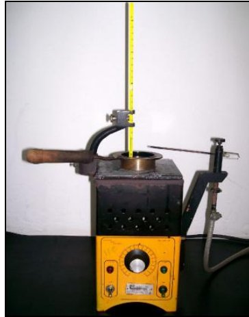
Figure 3. Equipment for determination of flashpoint
